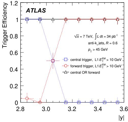
FIG. 5. Efficiencies for the central and forward jet triggers with a L1  $E_T$  threshold of 10 GeV, and for their logical OR, as a function of the rapidity  $y$  of the reconstructed jet in the transition region between the two trigger systems. The logical OR is used for the inclusive jet measurement to collect data in the  $2.8 \leq |y| < 3.6$  rapidity slice.
