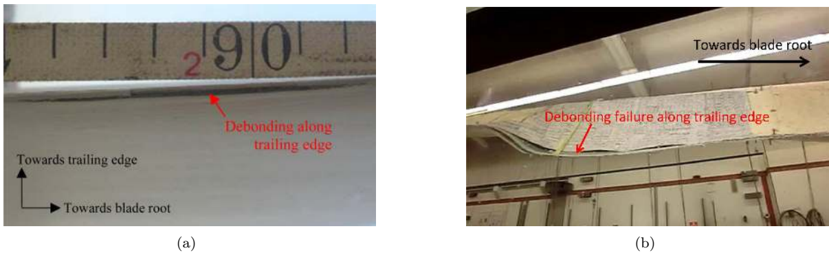
Figure 2: Typical debonding between pressure side and suction side shell at the trailing edge taken from [3]. The debonding along the trailing edge is depicted by the dark area on the shell (a). Local buckling induced trailing edge failure (b)
