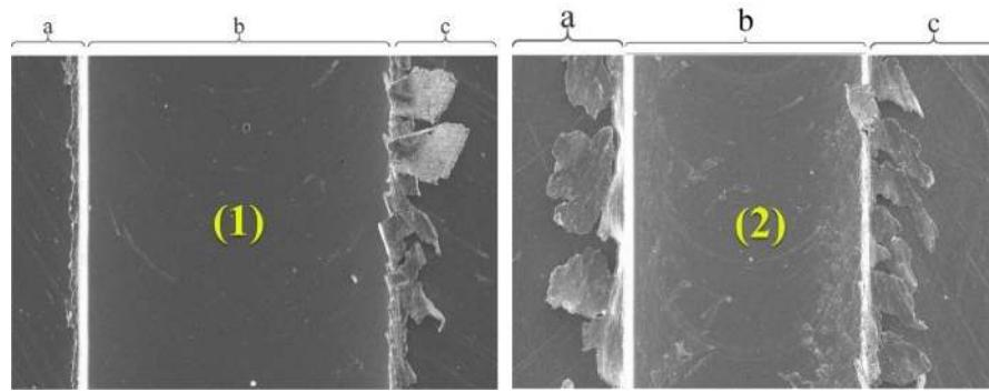
**Figure 4.** Slot and micro burr segmentation of sample (1) and sample (2): (a) micro burrs at the up milling side (left side), (b) slots, (c) micro burrs at the down milling side (right side).
