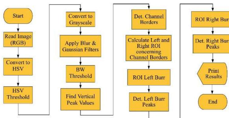
**Figure 3.** The flowchart of the measuring process.
