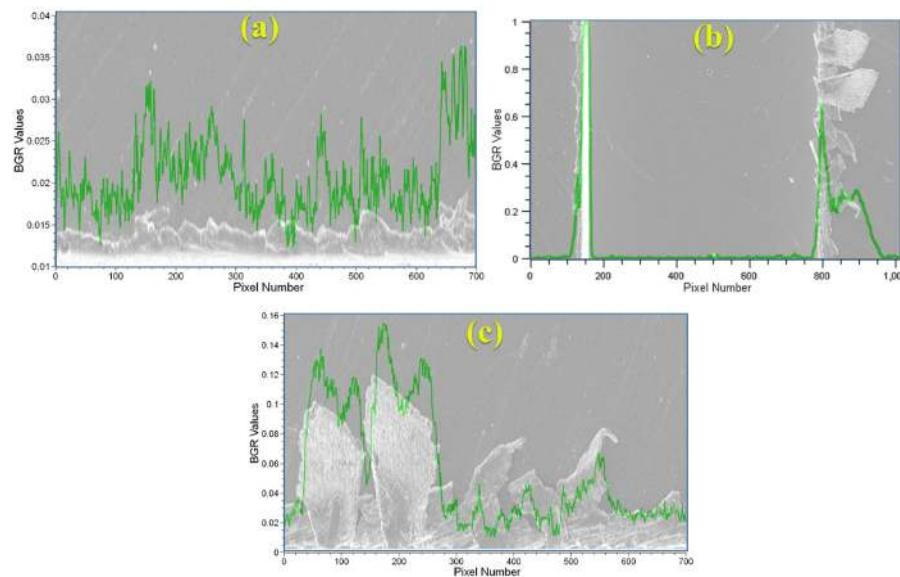
**Figure 5.** Sample (1): (a) automated burr measurement method at the up milling side according to the horizontal peak values, (b) automated measurement between the slot borders according to the vertical peak values, and (c) the automated burr measurement method at the down milling side according to the horizontal peak values.
