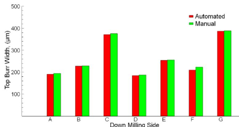
**Figure 10.** Automated and manual measurements of down milling sides.
