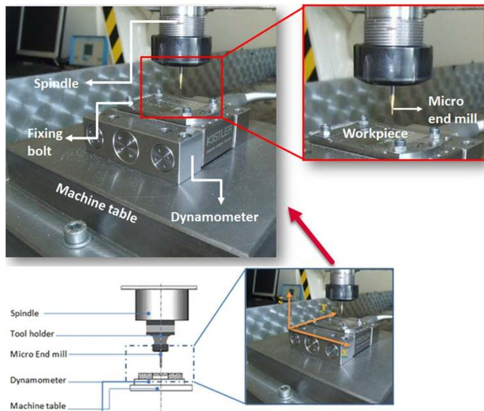
**Figure 1.** Experimental setup for the micro-milling process.
