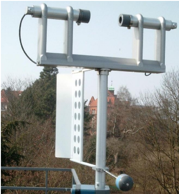
Fig. 1. The optical disdrometer ODM 470.
