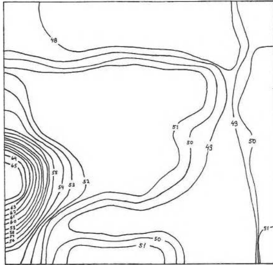
Fig. 12 Fault Finding. Influence of Removing Weatherstripping at 1600 Hz
