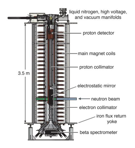
FIG. 2. A rendering of the aCORN apparatus indicating the major components and arrangement.
