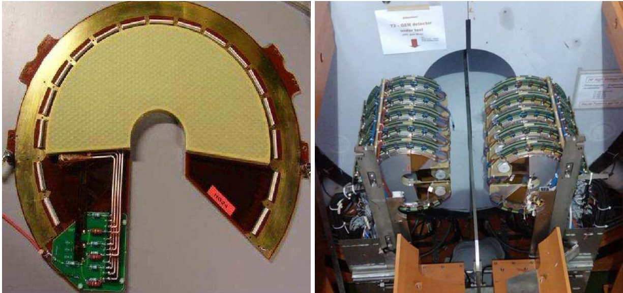
Figure 2.9: The TOTEM T2 telescope. Left: one detector plane. Right: installation of one arm in the CMS hadron-forward region.
