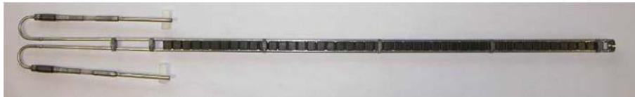
Figure 4.3: From [66]. The NuMI target.
