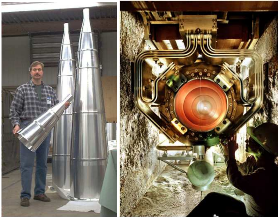
Figure 4.4: From [66]. Left: Photograph of inner conductors of the NuMI parabolic focusing horn. Right: Photograph of the first focusing horn.
