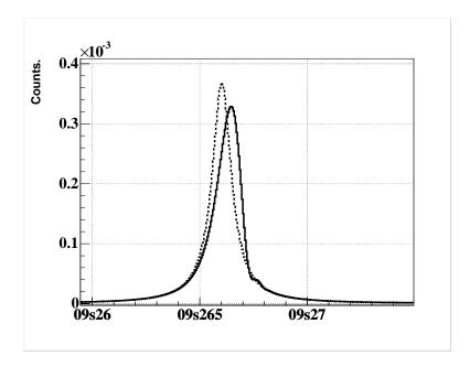
Fig. 8. Profile of the Airy peak without dynamical effects (dotted line) and with dynamical effects (full line) for a speed of  $10 \ \mu m/sec$ .
