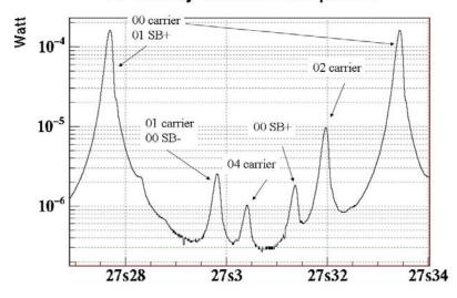
Fig. 10. Power transmitted by a free Fabry-Perot cavity.
