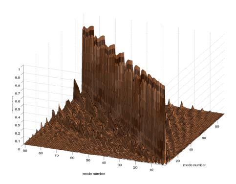
Fig. 3. Intensity reflection operator of the full interferometer with real maps. The modes are ordered {00,01,10,02,11,20,03,...}. Off-diagonal elements show coupling between modes inside the interferometer induced by surface defects. Diagonal elements slightly differ from unity mainly due to the finite size of the coatings.
