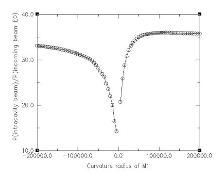
Fig. 11. Recycling gain of the sidebands as predicted by simulation as a function of the radius of curvature (in meters) of the power recycling mirror. The simulation is done for a simple cavity, the mirror transmissions are set respectively to 7.8% and 1.4% so that the expected gain corresponds to the maximum gain of the sidebands in Virgo (G=36).
