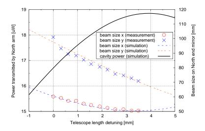
Fig. 7. Size of the beam after 3 km along two orthogonal axis as a function of the input telescope length tuning. The curves represents the result of the simulation while the dots are the experimental measurements. The wider black curve shows the power transmitted by the cavity as predicted by simulation.<sup>22</sup>
