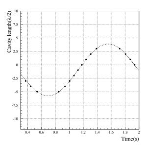
Fig. 9. Example of the measurement of the speed of the Fabry-Perot cavities: the dots represent the  $TEM_{00}$  peak positions and the line shows the length l(t) fitted to these points.
