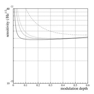
Fig. 2. Shot noise limited sensitivity as a function of the modulation depth for several values of sidebands transmission (T) and contrast defect (1-C):  $T=0.4,\ 1-C=10^{-5}$  (continous line),  $T=0.2,\ 1-C=3\times 10^{-5}$  (dashed line),  $T=0.1,\ 1-C=3\times 10^{-5}$  (dotted line) and  $T=0.1,\ 1-C=3\times 10^{-4}$  (dash-dotted line).
