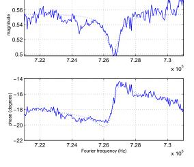
Fig. 6. Open loop transfer function of the lock of laser frequency on the cavity, around the frequency of the  $TEM_{02}$  mode (726 kHz). In blue, measured data; in red, the fitted curve.
