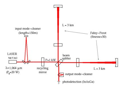
Fig. 1. Optical scheme of Virgo.
