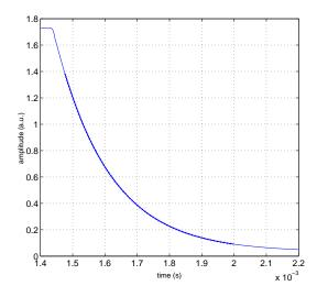
Fig. 5. Time decay experiment: power transmitted by the input mode cleaner, after a fast change of input laser frequency
