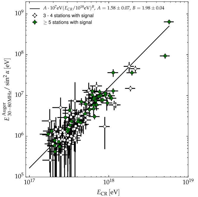
FIG. 2. Correlation between the normalized radiation energy and the cosmic-ray energy  $E_{\text{CR}}$  as determined by the Auger surface detector. Open circles represent air showers with radio signals detected in three or four radio detectors. Solid circles denote showers with five or more detected radio signals.
