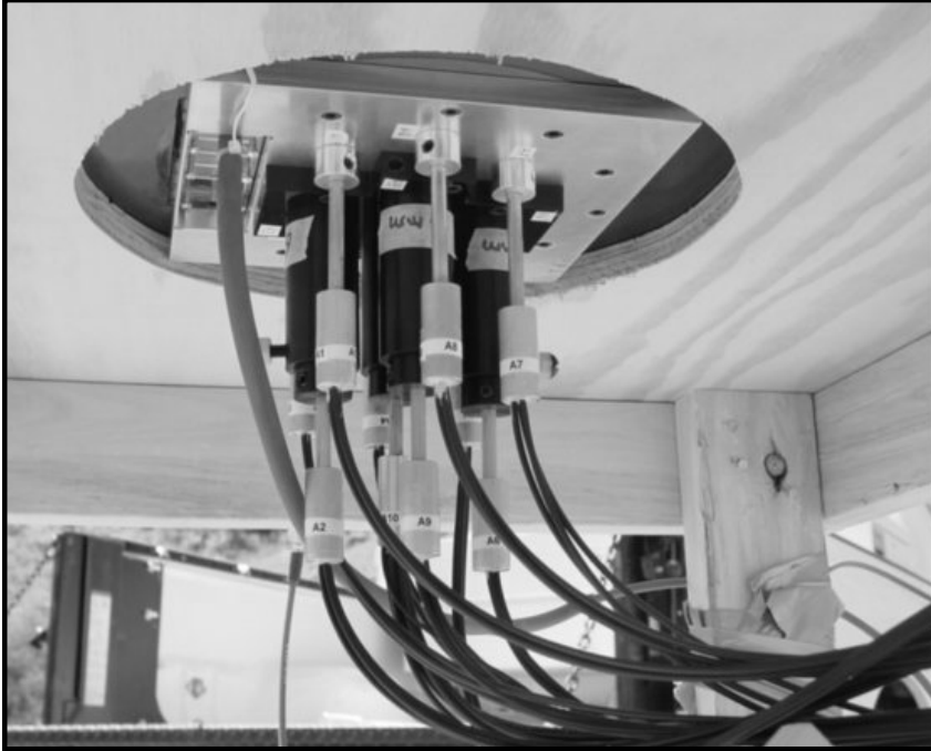
Fig. 6: Photograph of the diagnostic side of the target baseplate (facing down), in which all fiber probes are fielded and the argon gas is being circulated into the U_b -block.
