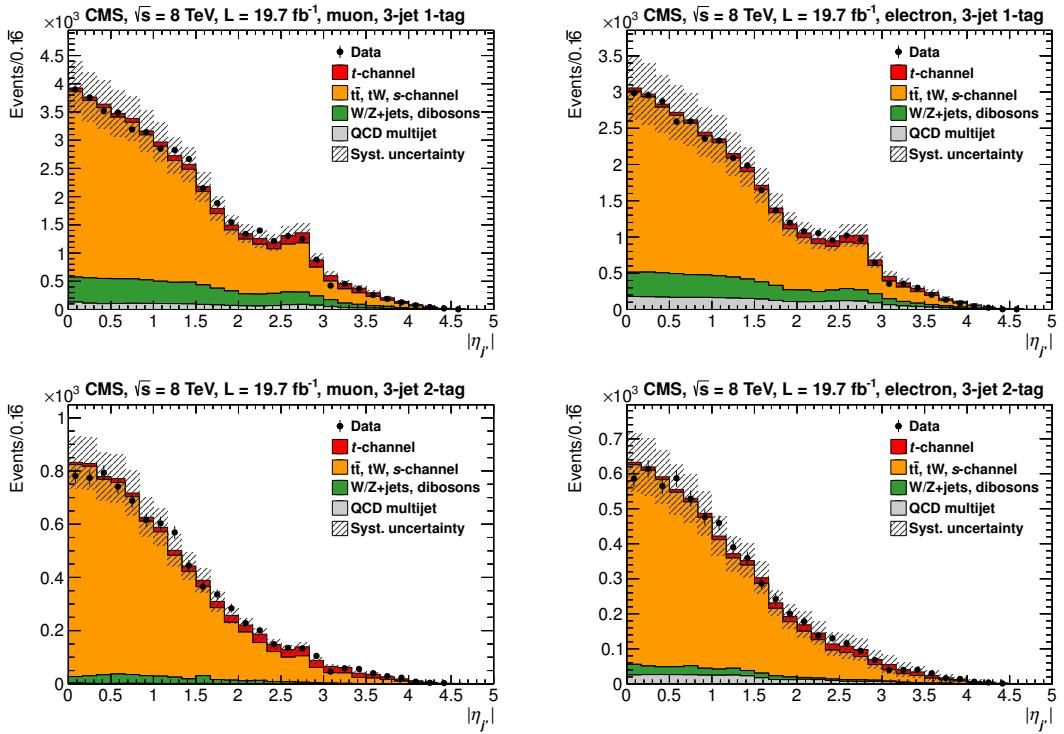
**Figure 2.** Distribution of  $|\eta_{j'}|$  in the 3-jet 1-tag (upper left, upper right), and 3-jet 2-tag (lower left, lower right) samples for muon and electron decay channels. The yield of the simulated processes is normalised to the results of the fit described in section 6. Systematic uncertainty bands include all uncertainties.
