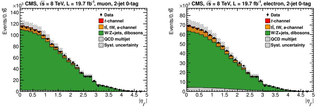
**Figure 5.** Distribution of  $|\eta_{j'}|$  in the 2-jet 0-tag sample for muon (left) and electron (right) decay channels. The QCD multijet contribution is derived from the fit to  $m_T$  and  $\cancel{E}_T$ . Systematic uncertainty bands include pre-fit uncertainties, both on the normalisation and on the shape of the distributions.
