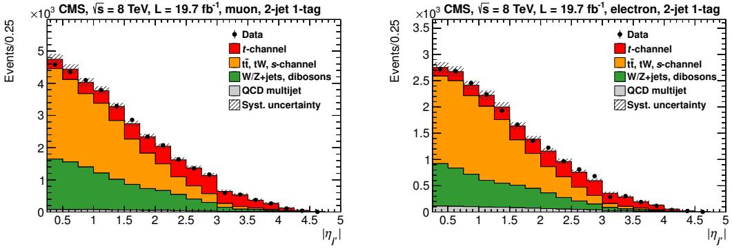
**Figure 8.** Fitted  $|\eta_{j'}|$  distributions for muon (left) and electron (right) decay channels, normalised to the yields obtained from the combined total cross section fit. Systematic uncertainty bands include the shape uncertainties on the distributions.
