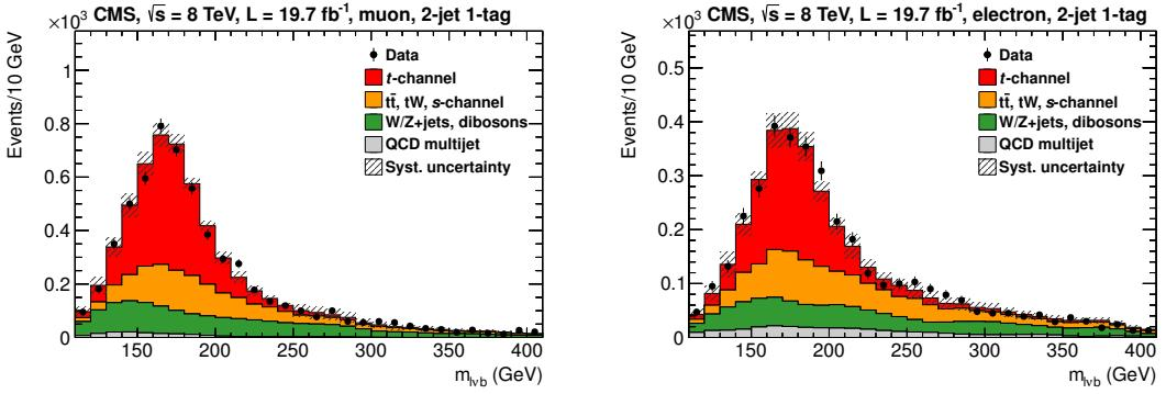
**Figure 10.** Distribution of reconstructed top-quark mass  $m_{\ell\nu b}$  for muon (left) and electron (right) decay channels, in the region with  $|\eta_{j'}| > 2.5$ , the contribution of each process is scaled to the cross section derived from the fit. Systematic uncertainty bands include the shape uncertainties on the distributions and uncertainties on the normalisation in the  $|\eta_{j'}| > 2.5$  region.
