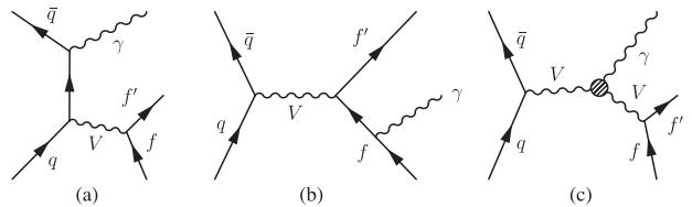
FIG. 1. The three lowest-order diagrams for  $V\gamma$  production, with  $V$  corresponding to both virtual and on-shell  $\gamma$ ,  $W$ , and  $Z$  bosons. The three diagrams reflect contributions from (a) initial-state radiation, (b) final-state radiation, and (c) TGC. The TGC diagram does not contribute at the lowest order to SM  $Z\gamma$  production, since photons do not couple to particles without electric charge.
