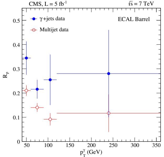
FIG. 5 (color online). The  $R_p$  ratio (described in text) as a function of the  $p_T$  of photon candidates for the barrel region of the ECAL in  $\gamma +$  jets and multijet data. The difference in  $R_p$  values for the two processes is attributed to the fact that jets in  $\gamma +$  jets events are dominated by quark fragmentation, while jets in multijet events are dominated by gluon fragmentation.
