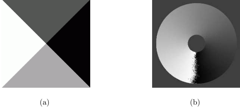
Figure 5: Disambiguation of the azimuth angle: (a) segmented image ( I_{quad} \in \{0, 1, 2, 3\} ), (b) image of the resulting azimuth angle \phi ( \phi \in [-\pi/2, 3\pi/2] ).
