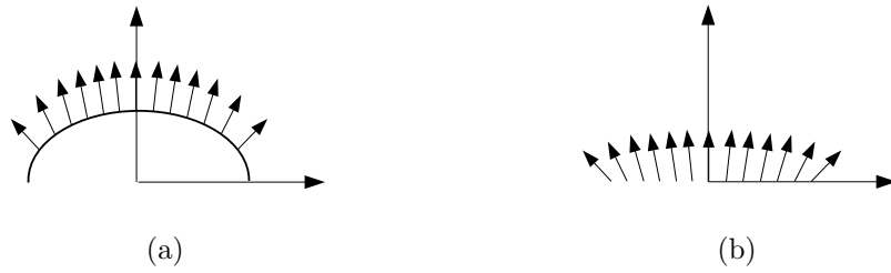
Figure 8: Three-dimensional parameters used: (a) normals \theta , \phi and surface height z , (b) only normals \theta , \phi (without integration process).
