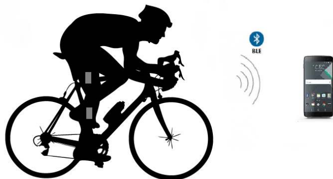
Figure 4.1: Architecture of the measurement system for cycling.
