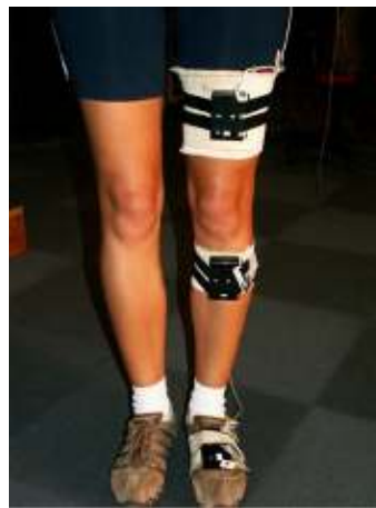
Figure 2.5: ProMove nodes placed in thigh, shank and foot of the subject [ Marin-Perianu et al., 2013 ].
