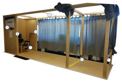
**Figure 7.** The evaluation prototype comprising (a) an introductory display and an RFID authentication device, (b) main display for user interaction, (c) the integrated aTUG chair with additional LBs, (d) a sensor belt including an inertial sensor, (e) light barriers at 3 m walking distance, (f) Intel RealSense D435 depth image camera placed approximately 4 m from the chair at an upper level facing onto it. Image originally published in [30].
