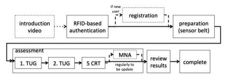
Figure 3. System's user-interaction workflow; incorporating user-interaction phases and assessments.
