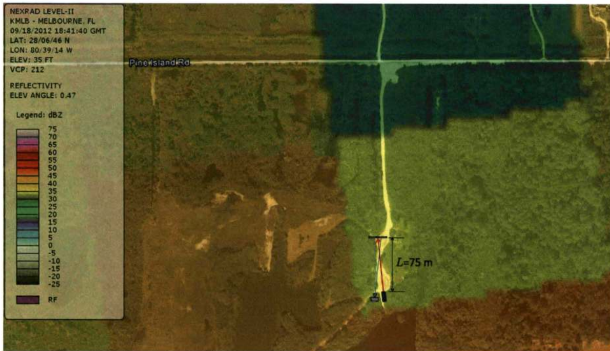
Figure 8. PES with 75 m distance to passive target, overlaid with September 18, 2012 Melbourne NEXRAD super-resolution data (250 m × 0.5°).
