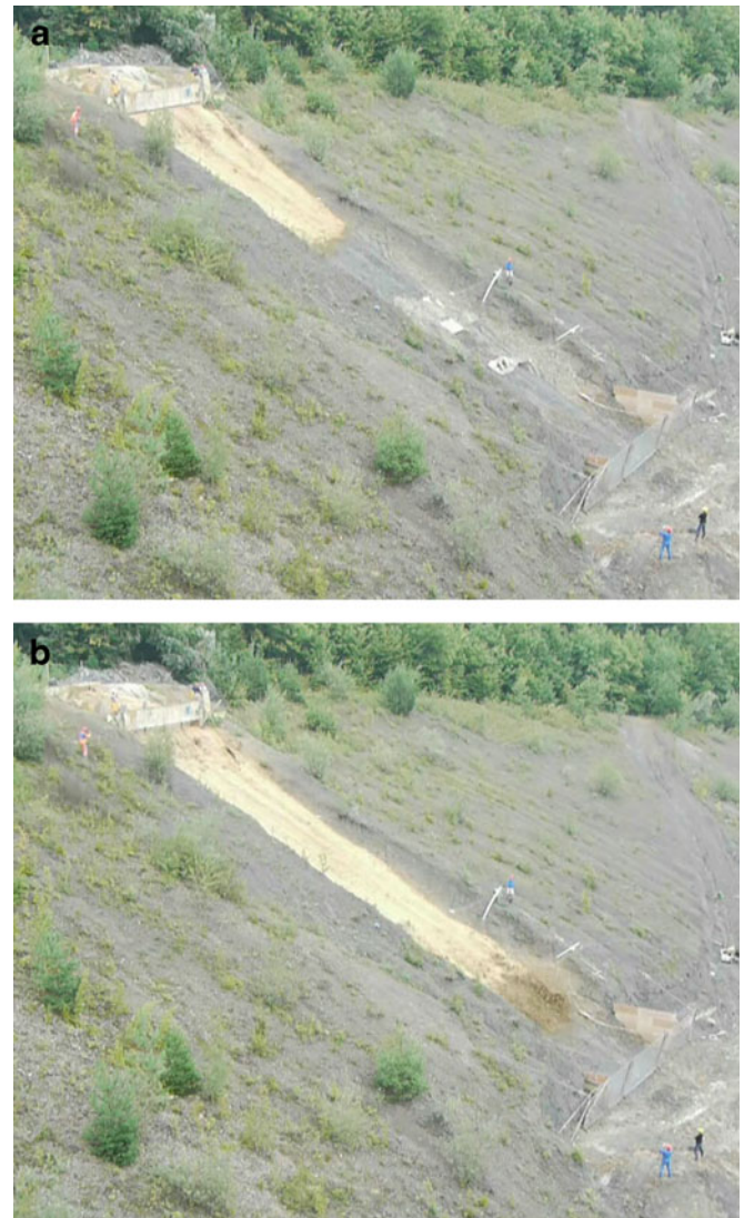
Fig. 2 Lateral view of release 15.1 just after release (a) and at the time of impact on the pressure plates (b)
