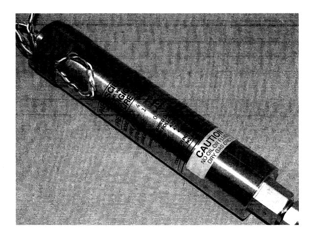
Figure 4.2 High-precision absolute pressure transducer used to measure the decaying pressure in the diffusion cell.
