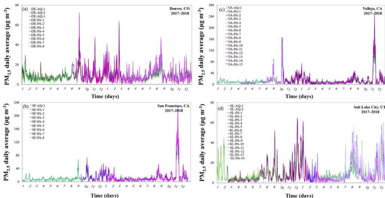
**Figure 3.** Time series of daily PM<sub>2.5</sub> measurements from the AQMS and PA-II units in each of the four areas: (a) Denver, (b) San Francisco, (c) Vallejo, and (d) Salt Lake City. Measurements from AQMS are represented by the green lines and the PA-II units are indicated by purple lines.
