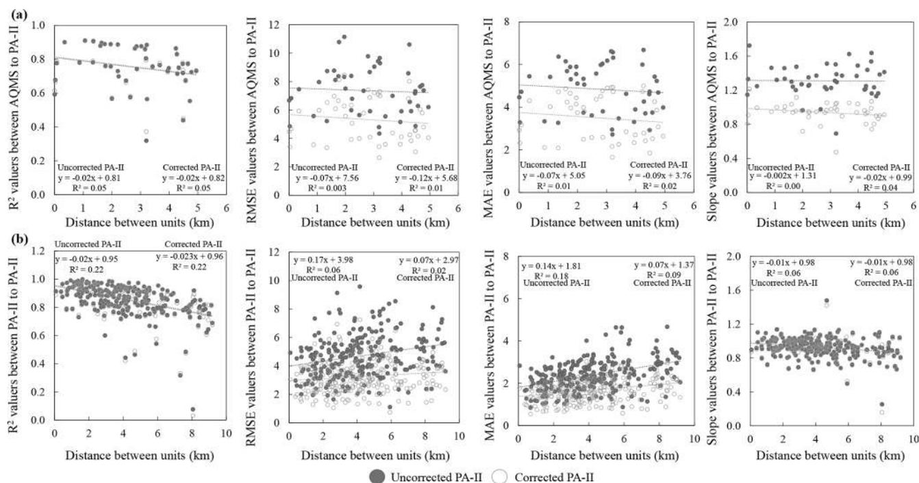
**Figure 7.** Comparison of distance (km) between PA-II and its nearest AQMS in all regions (a) and between each PA-II unit and all other PA-II units per region (b) for  $R^2$ , RMSE, MAE, and slope values received from the PM<sub>2.5</sub> hourly measurements comparison.
