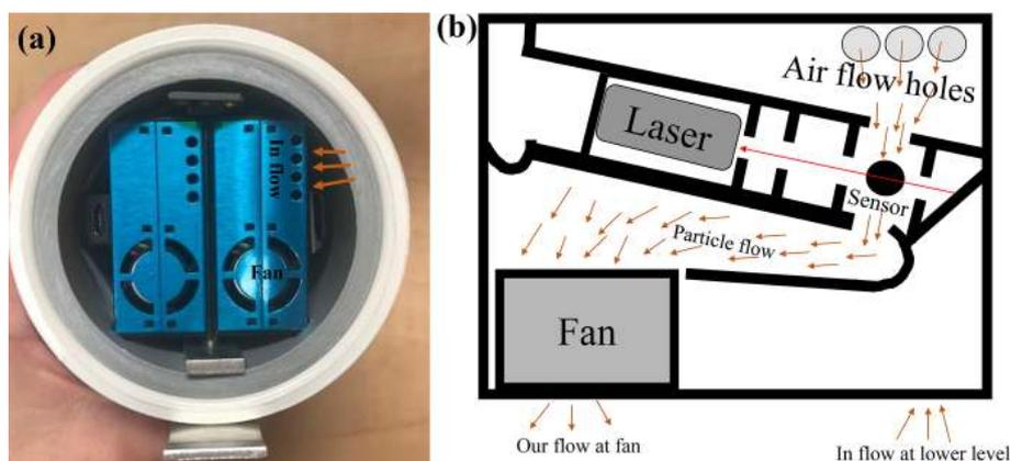
**Figure 1.** (a) Picture from the bottom of the PA-II unit containing two PMS5003 sensors (in blue). (b) Schematic of a single PMS5003 sensor. A fan draws the particles through the inflow (rounded holes) at the lower level of the sensor. The particles travel to the upper part of the sensor where they come out through the air flow holes and then pass through the laser path, causing the beam to scatter. Finally, the particles exit from the fan.
