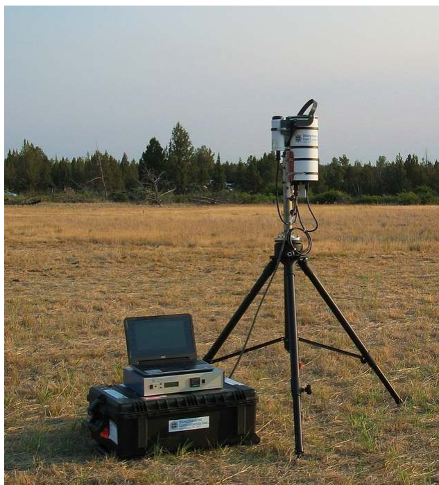
Figure 2. Setup of the GUVIS-3511 radiometer at Smith Rock State Park. The radiometer (white cylinder), BioSHADE assembly, and BioGPS are mounted on a tripod. Shown next to the instrument is the laptop for recording the data, the instrument's control unit, and a black case containing the power source.
