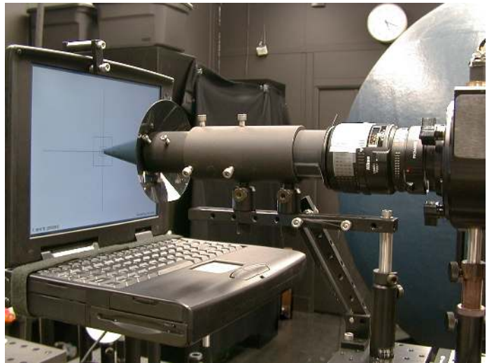
Fig. 2. The NFS is supported by two adjustable concentric tubes. A 120° apex gloss-black frustum surrounds the NFS to reduce reflections from the apparatus and light entering the tubing. The entire tubular assembly will swing away to permit an unobstructed view of the display by the camera.
