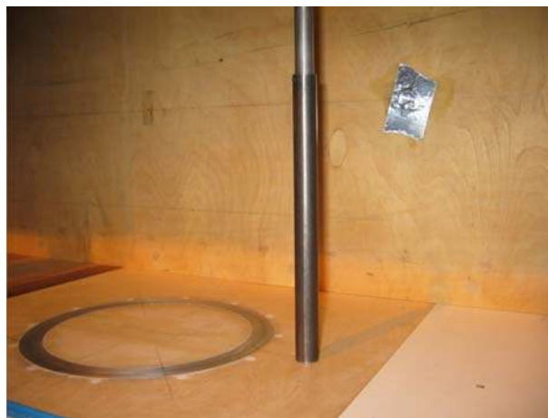
Figure 18. Photograph of the duct equipped with the bar upstream the rotating measurement disk
