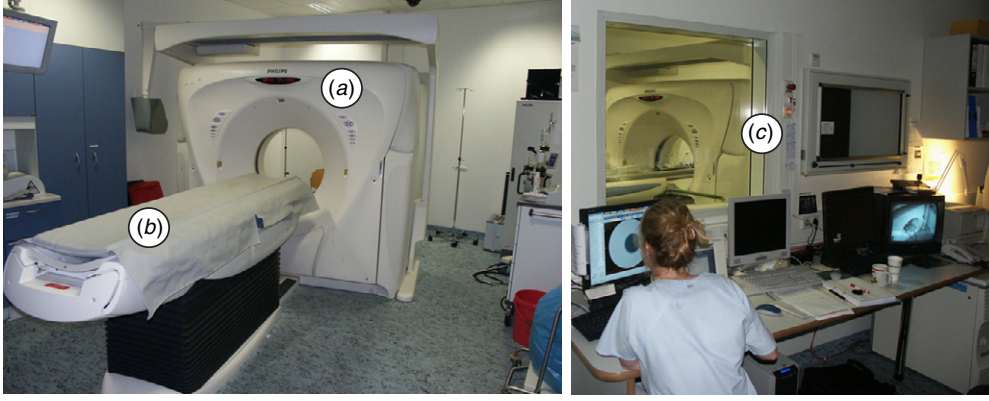
Figure 4. The CT system used: (a) gantry, (b) motorized platform, (c) control room.
