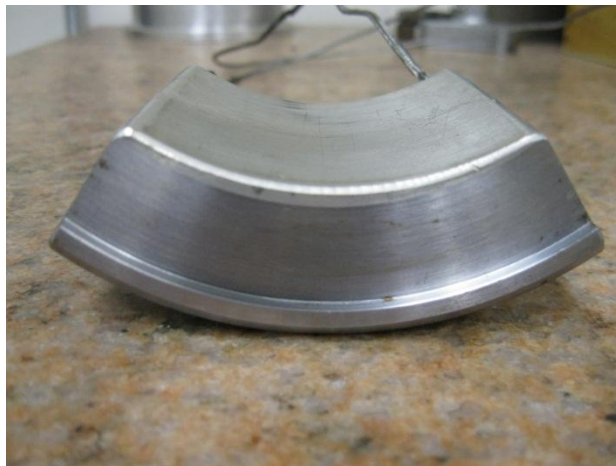
Figure 10: Test Bearing Pad
