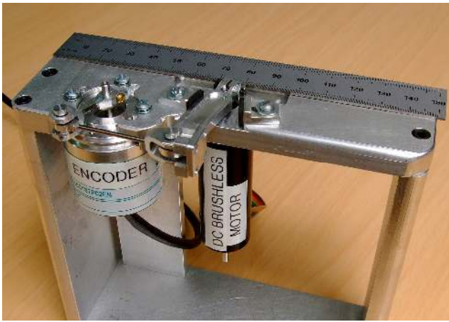
Figure 1: Photograph of haptic display used for these experiments, with ruler providing a size reference.
