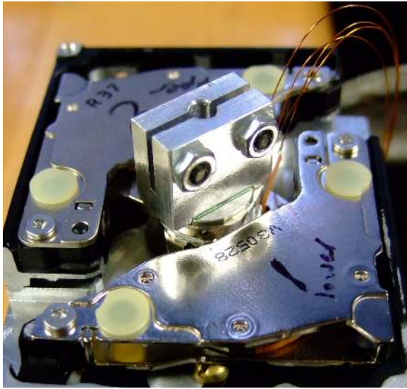
Figure 5: External Z-width probe to measure performance of haptic display. For size reference, the length of the long axis of the clamping block is approximately 10 mm.
