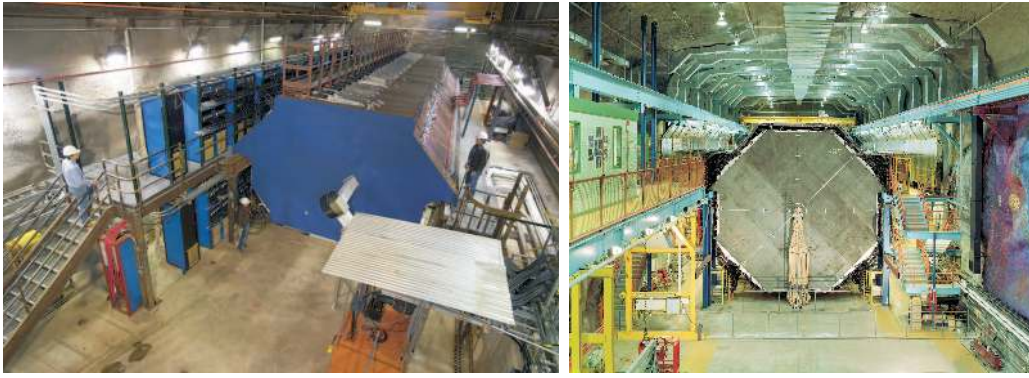
Figure 3.6: The MINOS near (left) and far (right) detectors.
