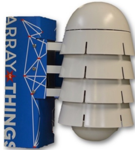
Fig. 2 An AoT node. Computers, camera, and light (Ultraviolet (UV), Infrared (IR), and visible) sensors are in the blue enclosure; a cellular modem, camera, environmental (vibration, sound, magnetic field, temperature, relative humidity, and barometric pressure), and air quality (CO, NO 2 , SO 2 , PM2.5, and O 3 ) sensors are in the white enclosure.
