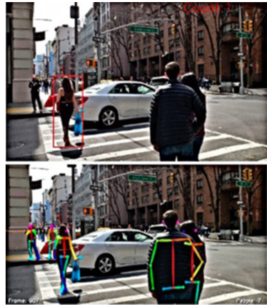
Fig. 6 Use of edge computing in Ref. [53] to detect a pedestrian crossing during a red-light (top) and analyze body language (bottom). Images courtesy of Potdar and Torrens, used with permission.
