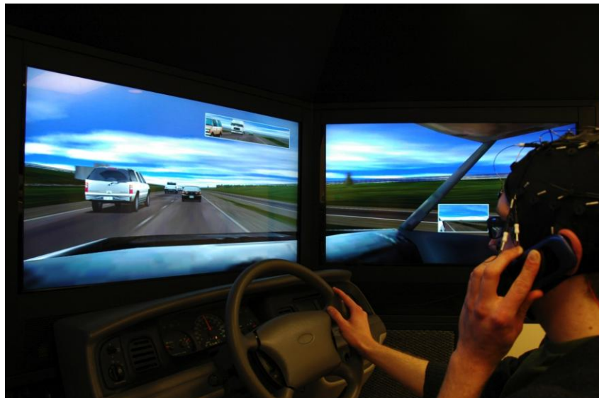
Figure 22. Image of the L3 Patrol-Sim driving simulator with a subject using a hand-held cell phone.
