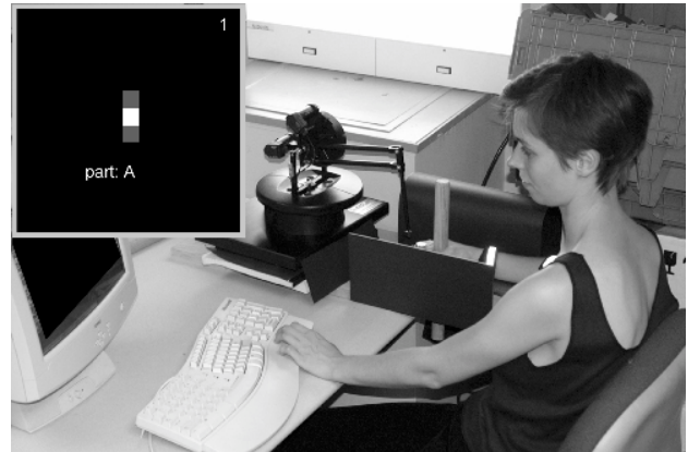
Figure 1. The experimental setup. Subjects sampled pairs of forces with their right index finger by pressing against virtual "springs" simulated by the PHANToM TM device. The image on the computer display (here, in the top left) indicated when the subject had pressed against the springs to a target position. During each run, subjects' hands were shielded from view with an opaque sheet of black paper.
