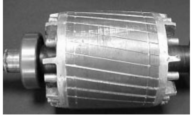
Fig. 2. Rotor of a 0.75-kW induction machine used for the test.
