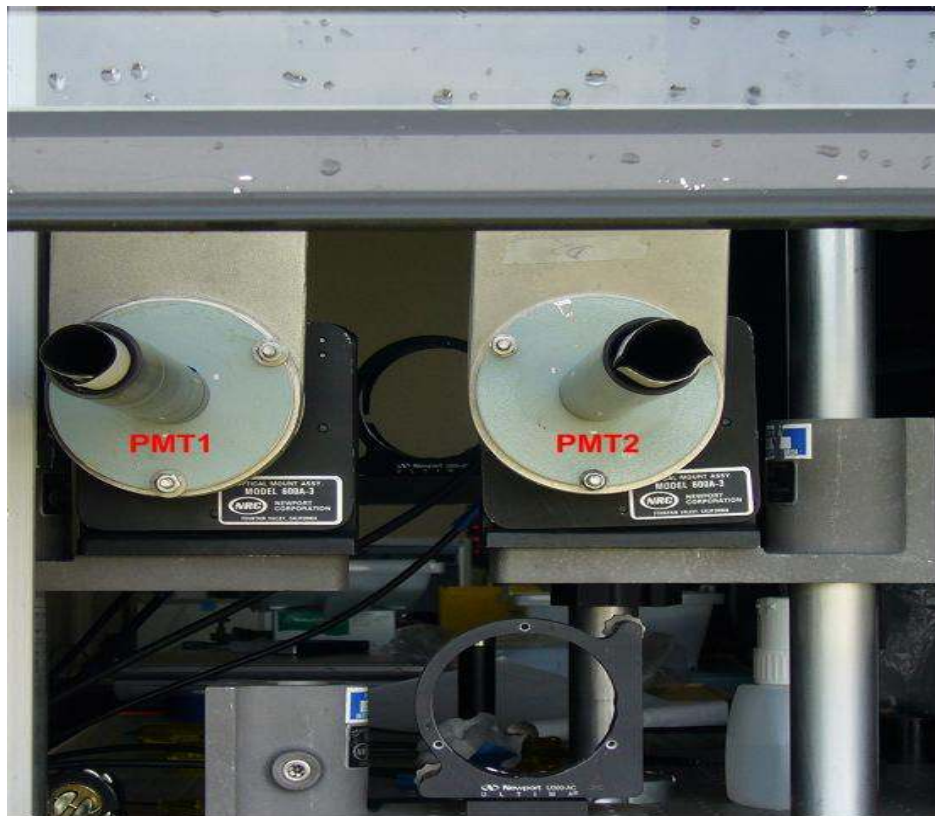
Figure 14: PMT configuration for crosswind speed data collection.
