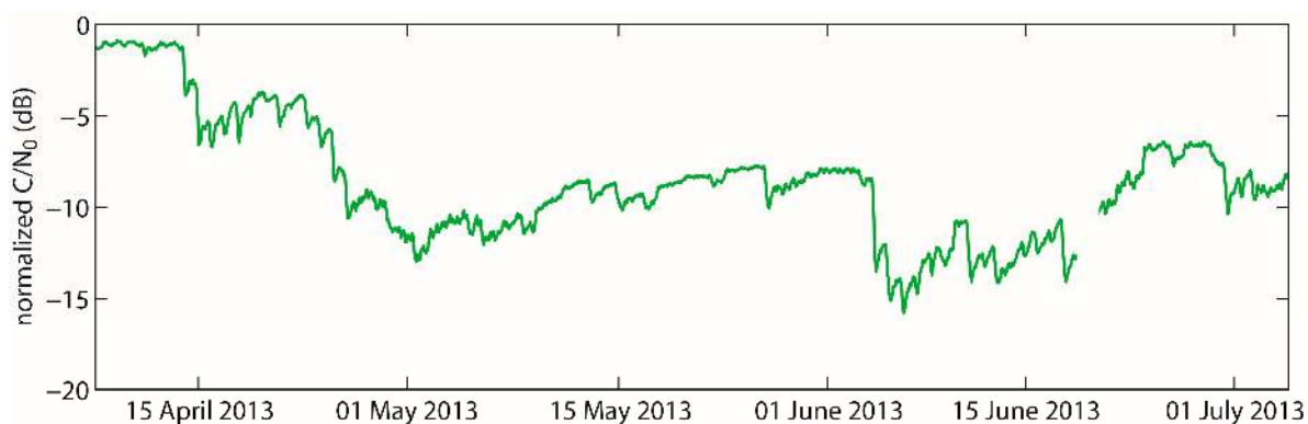
Figure 6. Normalized GPS C/N_0 values (dB) taken as the mean of the two GPS receivers under the snow cover (GPS2 and GPS3) at the Weissfluhjoch test site for the period 7 April–6 July 2013.
