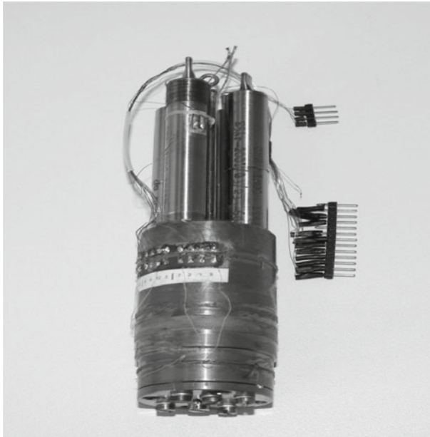
Fig. 2 IMGC model of multicompartiment cell for realization of gaseous fixed points of ITS-90
