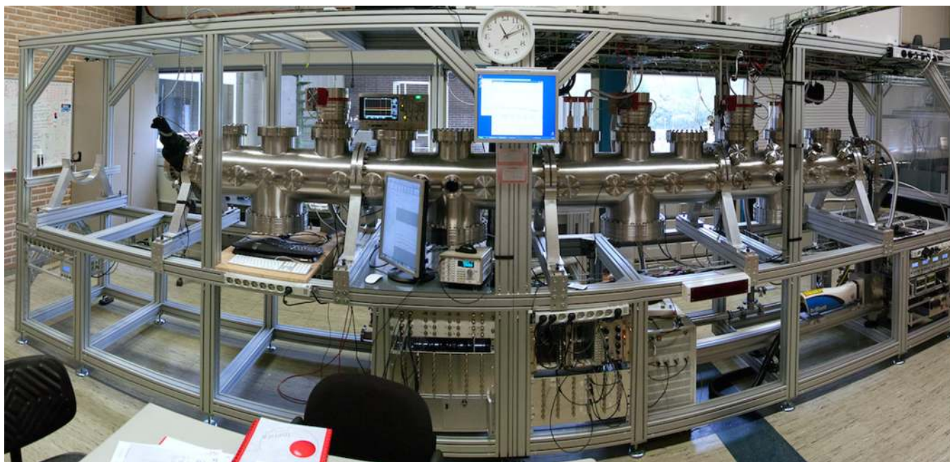
Fig. 4. Panoramic view of the Stark decelerator, operational at VSI in Groningen. This device, with a length of 4.5 meter, was built with the purpose of studying fundamental symmetry violations (note the clock) with slows beams of heavy diatomic molecules.
