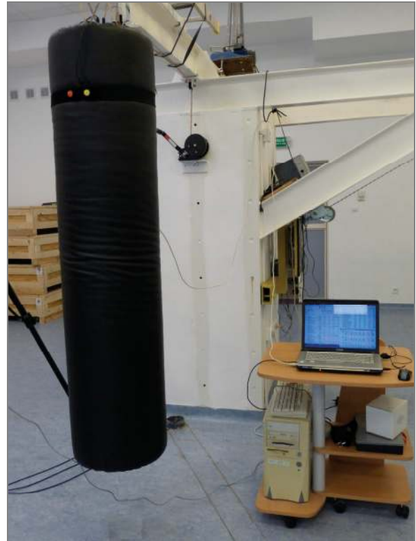
Fig. 1. BTS-4AP-2K dynamometric punching bag with an embedded accelerometer
