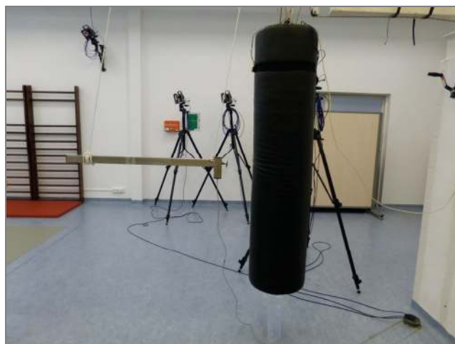
Fig. 4. The view of the dynamometric punching bag having an embedded accelerometer when delivering test strike
