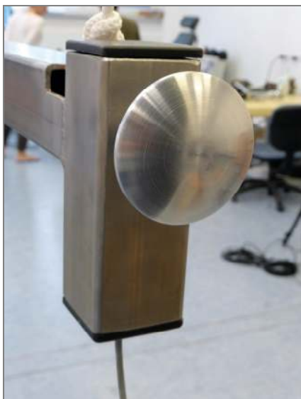
Fig. 5. The view of the impact hammer's spherical face used to deliver test strikes
