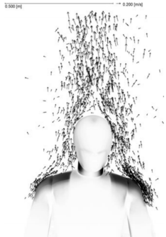
Fig. 6. Particle tracks of the upward flow of the thermal plume. The tracks are already converted into vectors indicating the direction and speed of the airflow (room temperature: 18°C)
