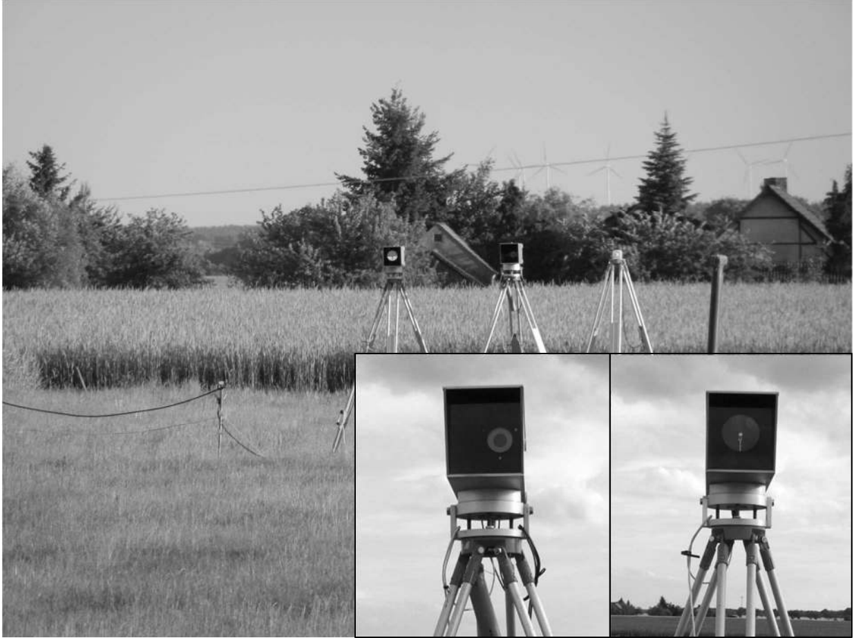
Figure 4.2: Field set-up of the scintillometer experiment in Falkenberg with a close-up of the modified large-aperture scintillometers from Wageningen University.
