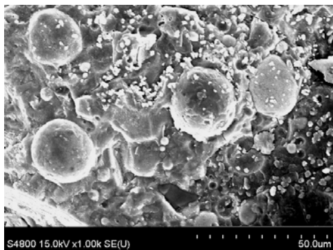
Fig. 8. SEM image of AASF mortars with fly ash/slag ratios of 50/50 (MFS) at the liquid/binder ratio of 0.5 at the age of 28 days at 1K x.
