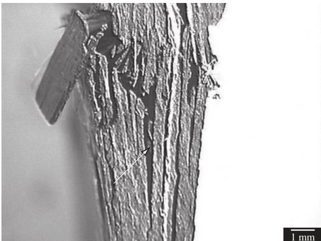
Figure 9. 8552/8HS laminate after the compressive test.
