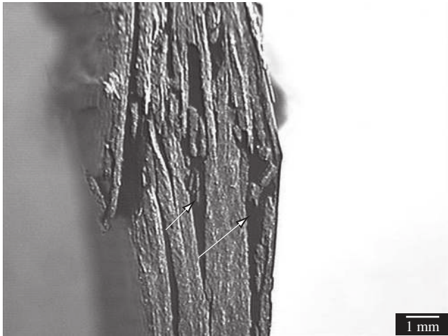
Figure 8. F584/PW laminate after the compressive test.
