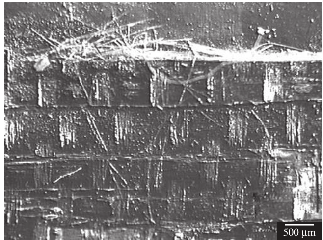
Figure 10. Typical aspect of a 8552/8HS laminate specimen after compressive test.
