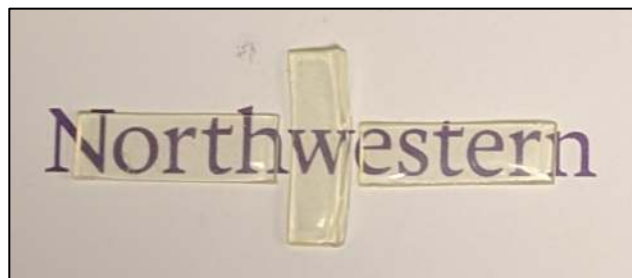
Figure 3. Photograph of Block-66 . Each sample is approximately 20 x 6.5 x 0.5 mm.
