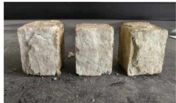
Fig. 4 Compressive strength samples after testing
