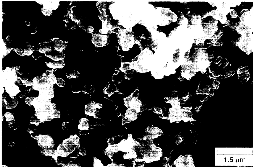
Figure 19b - Detail Of Cu-8 Cr-4 Nb Fracture Surface (Extrusion L-3107 Tested At 500°C/84.0 MPa)
