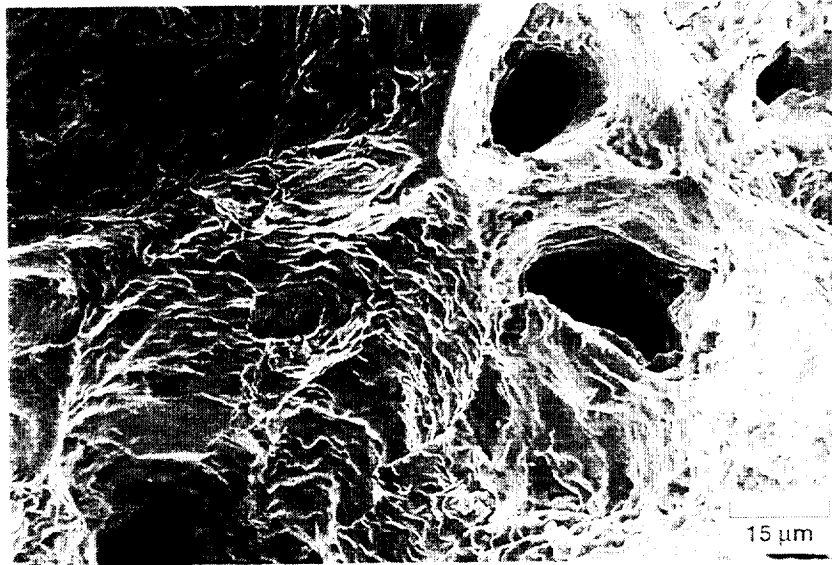
Figure 19d - Typical Fracture Surface Of NARloy-Z Creep Samples (Plate 3 Tested At 800°C/10.4 MPa)
