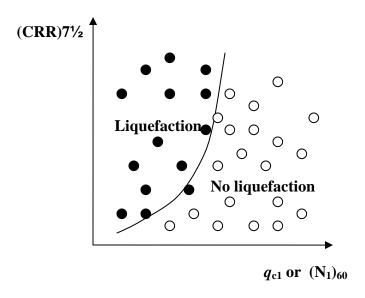
Figure 4 – Semi-empirical approach to evaluate liquefaction resistance.
