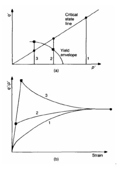
Figure 5 – Idealized behavior of cemented soils: (a) stress paths; (b) stress-strain behavior (After Coop and Atkinson 1993)
