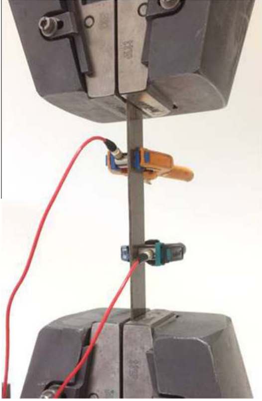
Fig. 1. Composite specimen with acoustic emission sensors. (For interpretation of the references to color in this figure legend, the reader is referred to the web version of this article.)
