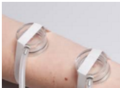
Figure 4: Circular aperture of the dome used to elevate the skin in suction test.
