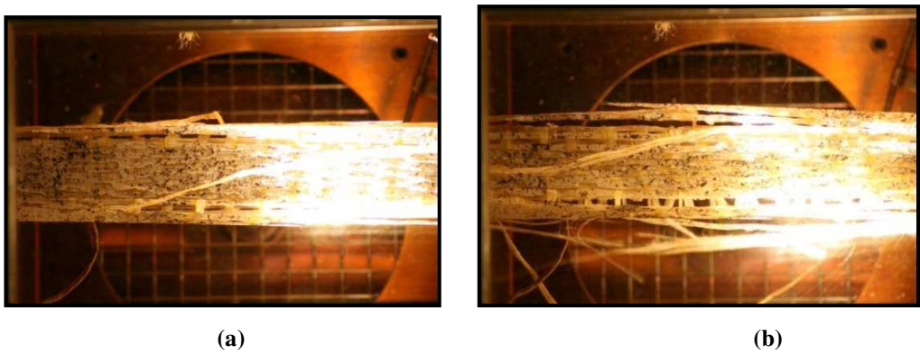
Figure 10: Failure of GFRP tensile coupons at 200°C (a) just before failure, and (b) just after failure (photos rotated 90° clockwise)
