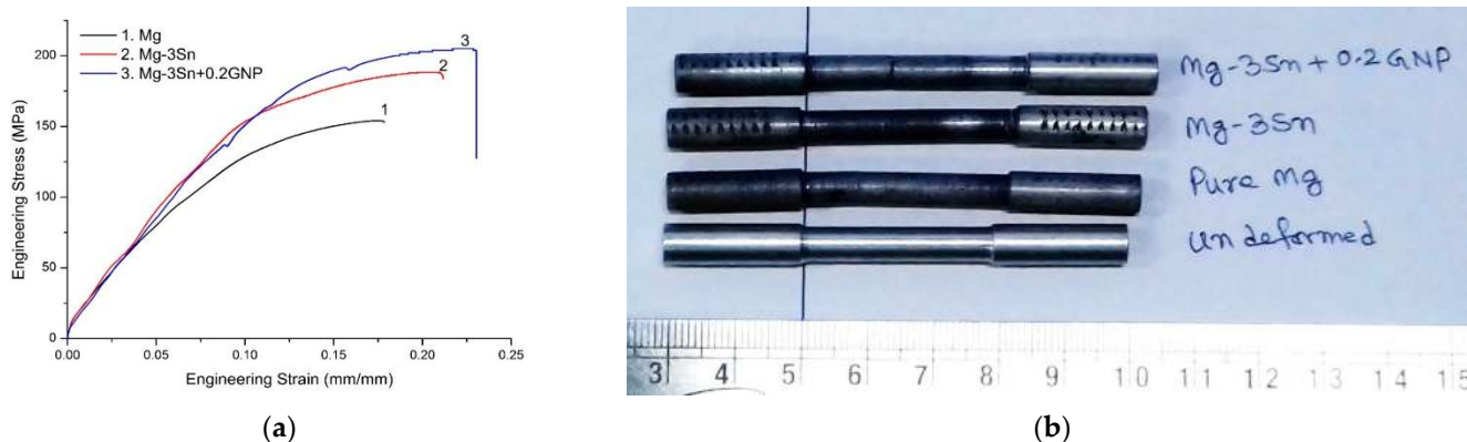
Figure 8. Tensile behavior of pure Mg, Mg-3Sn alloy, and Mg-3Sn + 0.2 GNP composite: (a) representative tensile engineering stress–strain curve and (b) corresponding images of undeformed and deformed tensile samples.
