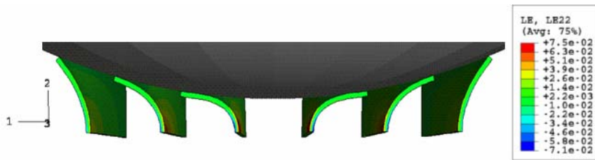
Figure 6. FEM simulation shows the deformation of the nanolines with 220 nm indentation displacement indentation on SiNLs.
