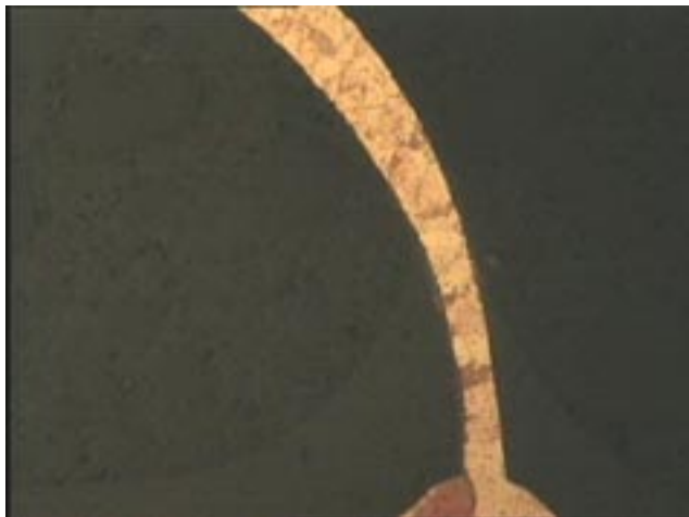
Figure 12 Microstructure of Heat affected zone showing grain size distribution (500X)
